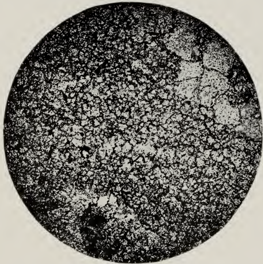
FIG. 33. Photomicrograph (natural light) of the same field shown in figure 32, showing the outlines of the original calcite grains which are now largely replaced by fluorite. (After Bain, H. Foster, Fluorspar deposits of southern Illinois: U. S. Geological Survey Bull. 255, Pl. VI-A, 1905.)
